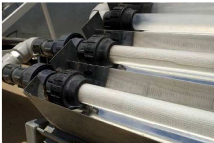
Fig. 2. Scheme of the supported \text{TiO}_2 configuration (left). View of the supported photocatalyst into the glass tubes of the CPC photoreactor (right).
